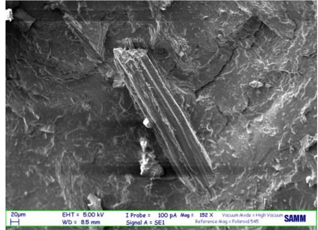
The pictures below showed a comparison between composites processed with two different screw configurations. In the picture on the left is evident a poor mixing quality of kenaf while the other picture the filler is well distributed and dispersed thanks to a modified screw configuration.
