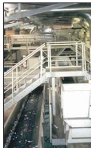
A system of fast-moving c separates bottles by resin color and removes tramp before conveying material balers.
