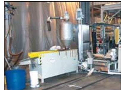
**AFTER:** Washed and separated resin is extruded into gray and black PE compounds for furniture, car parts, pipe, and film.
